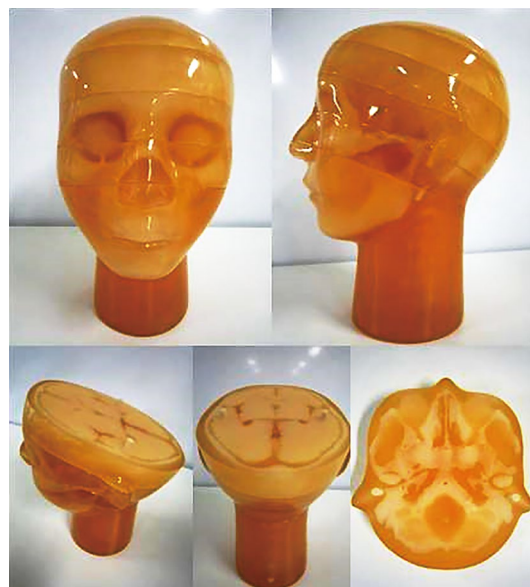
Figure 3 The picture of the X-ray CT measurement phantom to evaluate brain.
